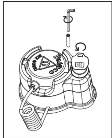
③ Insert the key and unlock it, screw the set screw into the right hole by a 2mm Allen key.
