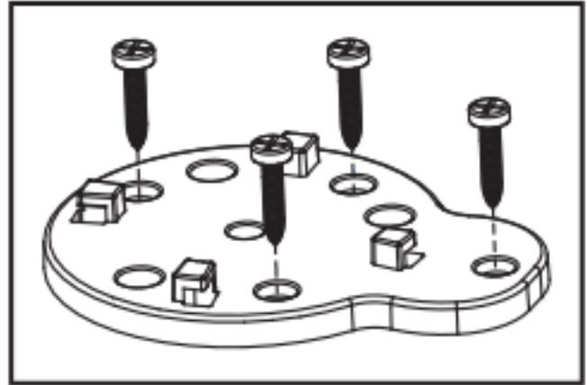
① Screw the four screws into the desktop through the holes of section 2
