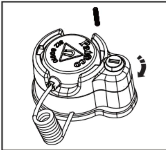
② Put the whole ejector on top of section 2, then turn it in the direction of the arrow to fasten.
